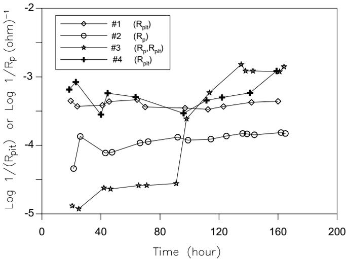
Fig. 6. Time dependence of  $R_p$  or  $R_{pit}$  for four different tests.
