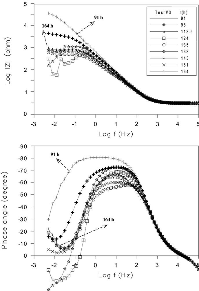
Fig. 3. Bode plots for Al 2024 exposed to AS containing *B. subtilis*, addition of antibiotics after 90.5h.
