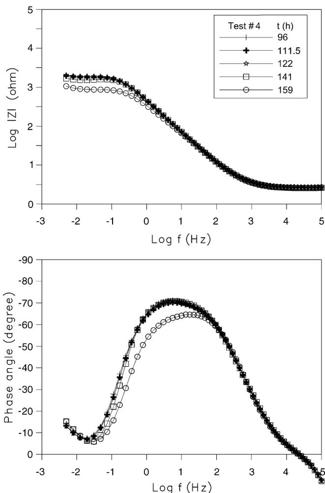
Fig. 4. Bode plots for Al 2024 exposed to sterile AS, addition of antibiotics after 90.5h.
