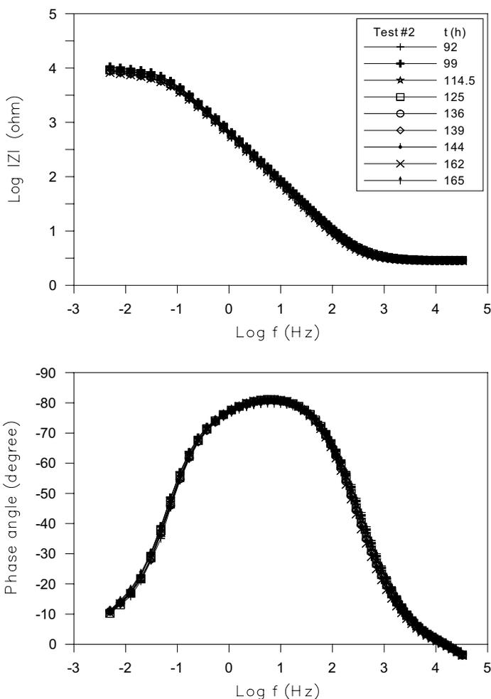
Fig. 2. Bode plots for Al 2024 exposed to AS containing *B. subtilis*.
