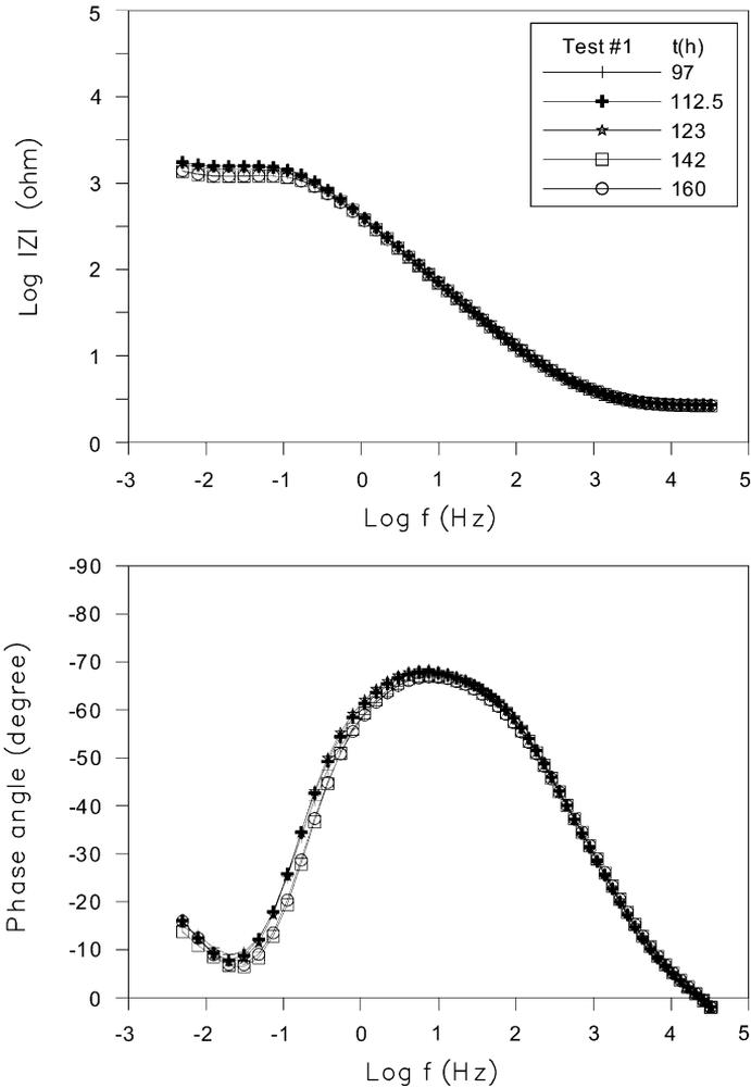
Fig. 1. Bode plots for Al 2024 exposed to sterile AS.
