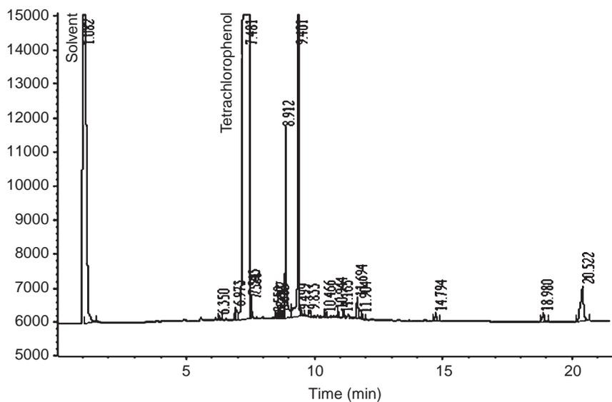
**Fig. 4** Gas chromatograph of the PED-treated 2,3,5,6-TeCP solution after 24 h processing with acclimated activated sludge
