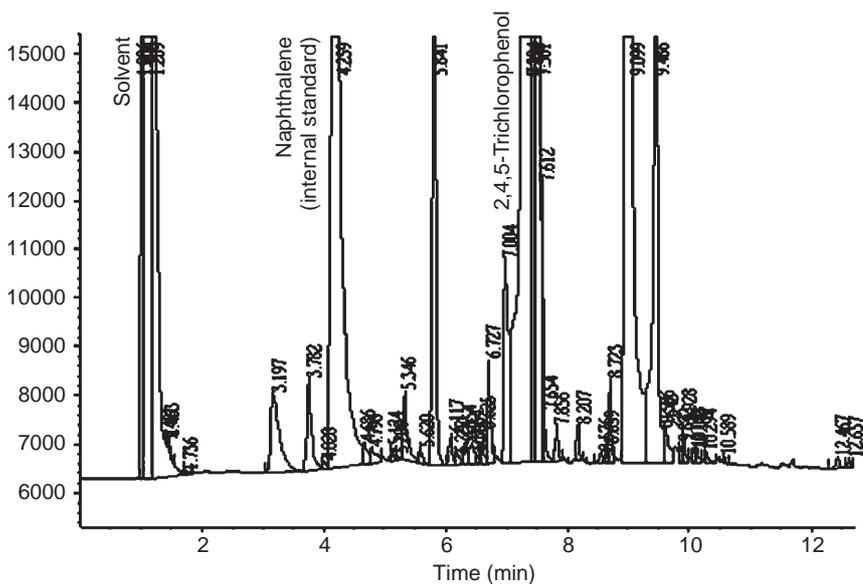
**Fig. 2** Gas chromatograph of the PED-treated 2,4,5-TCP solution after 24 h processing with acclimated activated sludge. The 2,4,5-TCP and internal standard naphthalene peaks are labeled
