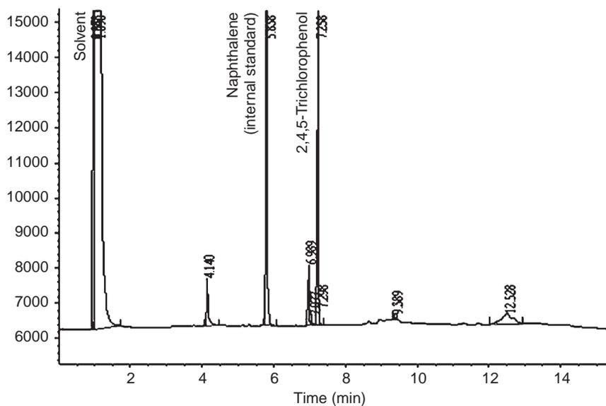
**Fig. 3** Gas chromatograph of 100 ppm 2,3,5,6-tetrachlorophenol (2,3,5,6-TeCP) after processing in the PED reactor
