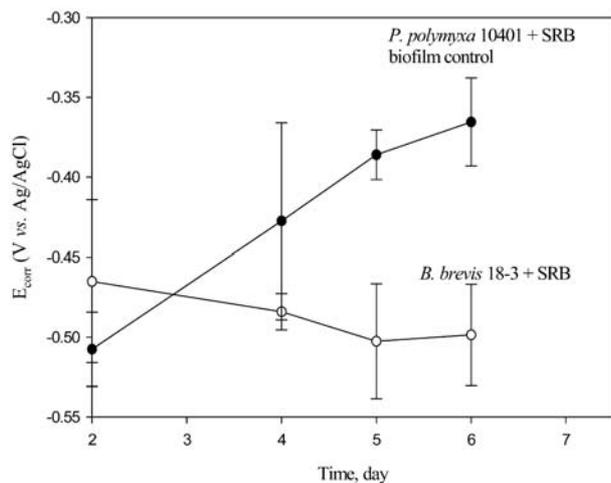
**Fig. 3** Corrosion potential ( $E_{corr}$ ) of mild steel 1010 in the presence of SRB (*D. orientis*) and *B. brevis* 18-3 (protective) or *P. polymyxa* 10401 (control) biofilms in continuous reactors containing Baars' medium. Solid symbols represent *P. polymyxa* 10401 + SRB (duplicate), open symbols represent protective biofilm of *B. brevis* 18-3 + SRB (duplicate). Error bars shown for the standard deviations
