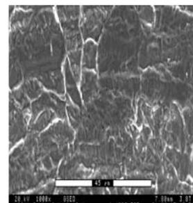
(b) Mild steel 1010 exposed to *D. orientis* in the presence of the supernatant of *P. polymyxa* 10401 culture which did not contain gramicidin S in Baars' medium in the batch experiment
