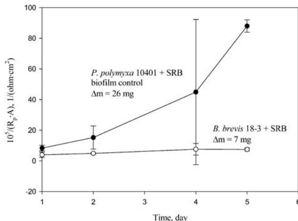
**Fig. 4** Relative corrosion rates [ $1/(R_p A)$ ] for mild steel 1010 in the presence of SRB (*D. orientis*) and *B. brevis* 18-3 (protective) or *P. polymyxa* 10401 (control) biofilms in continuous reactors containing TMI water. Symbols and error bars as defined in Fig. 3. Mass loss shown after 5 days.
