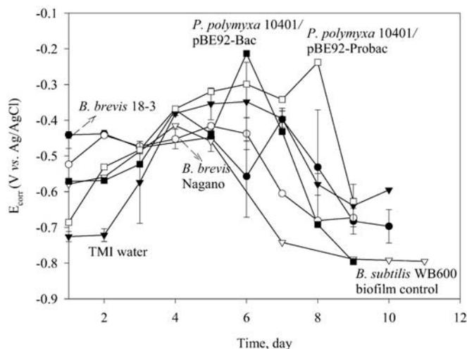
**Fig. 7** Corrosion potential ( $E_{\text{corr}}$ ) of mild steel 1010 in the presence of SRB (*D. vulgaris*) and the single biofilm of *B. brevis* 18–3, *B. brevis* Nagano, *P. polymyxa* 10401–pBE92–Probac, *P. polymyxa* 10401–pBE92–Bac, or *B. subtilis* WB600 in continuous reactors containing TMI service water. TMI service water without protective biofilm was also used as a negative control. Symbols and error bars as defined in Fig. 6
