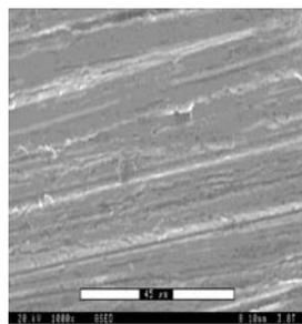
(a) Mild steel 1010 exposed to *D. orientis* in the presence of the supernatant of *B. brevis* 18-3 culture which contained gramicidin S in Baars' medium in the batch experiment
