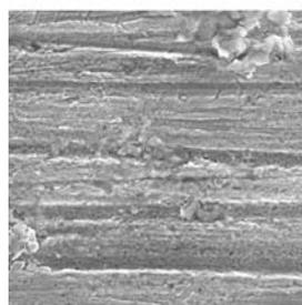
(c) Mild steel 1010 exposed to *D. vulgaris* in the presence of *B. brevis* 18-3 biofilm which produced gramicidin S in TMI water in the non-simultaneous continuous experiment
