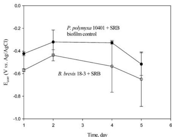
**Fig. 5** Corrosion potential ( $E_{\text{corr}}$ ) of mild steel 1010 in the presence of SRB (*D. orientis*) and *B. brevis* 18-3 (protective) or *P. polymyxa* 10401 (control) biofilms in continuous reactors containing TMI water. Symbols and error bars as defined in Fig. 3
