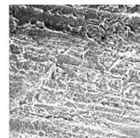
(d) Mild steel 1010 exposed to *D. vulgaris* without protective biofilm in TMI water in the non-simultaneous continuous experiment
